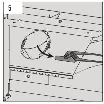
Hold the smoke outlet connector (which has already been connected to the duct) by the handle and attach it to the stove [figures 1 & 3]
