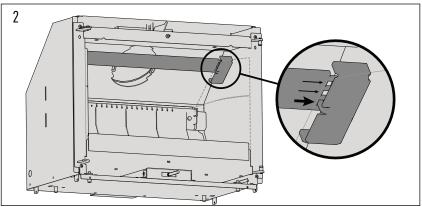
The default position of the vermiculite deflector housing is the highest position. If you have a "lazy'" chimney, you can lower the housing to the second or third notches (figure 2).
