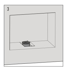
Install the air inlet duct and attach the nozzle with a metal duct clamp.
